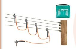
LV Earthing Kits can be applied by hand using the S9B Long Handle clamps. Kits can be provided for up to 5 cables (three Phase, Neutral and Earth Line End clamps), and are supplied including a heavy duty pvc carry bag for protection of the equipment. The length of the 50sqmm leads is usually 1.5m, although these can be made to any length/colour depending upon requirements. Part Numbers: MISC-00029 (With pvc bag)
