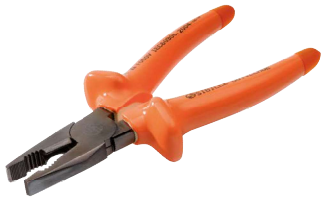
Insulated all-angle pliers MS4-185 NF EN 60900/IEC 60900/NF ISO 5743/NF ISO 5744/NF ISO 5746 SPECIFICATIONS • Length: 185 mm • Weight: 320g
