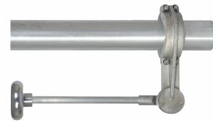
The machined clamp is supplied in two halves that are bolted together around the busbar using the supplied fasteners. A 38mm diameter spigot and corona shield, common to all spigot clamps and busbar sizes, is then
